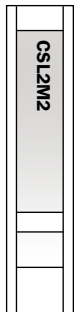
2 3/4" stiles, 6 1/2" top rail & 12" bottom rail with 5 5/16" intermediate rail 23 3/4" from bottom of panel
